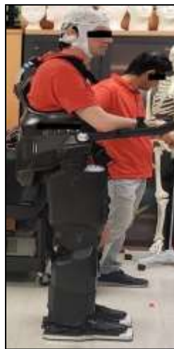
Figure-6 Typical BCI controlled Exoskeleton setup
